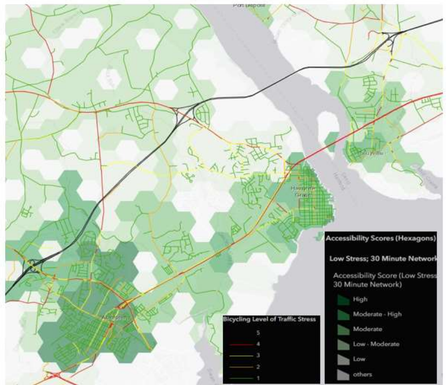
Data Source: MDOT Bicycle Accessibility Map Application, 2023. This interactive maps shows the Level of Stress for on-road cyclists, one tool for analyzing opportunities.
